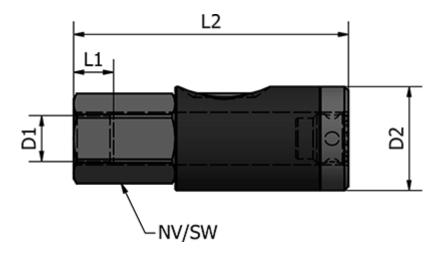
D1 = G 1/2D2 (mm) = 26 L1 (mm) = 11 L2 (mm) = 77.5 SW (mm) = 24 Weight (g) = 150
